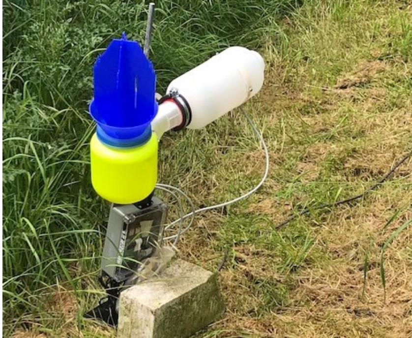
Photo by LIST of a DiMON device connected to a Vane Trap
